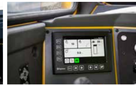
Scooptram ST14 has an intelligent control system featuring traction control speed limiter, overspeed protection and automatic ride control.
