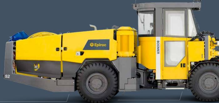
The filtration package provides longer life on rock drills, hydraulic valves and pumps which leads to lower running costs Carrier improvements include new frames with stronger waist, faster tramming, less breakdowns and new stronger diesel engines up to stage 4F
