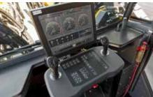
The control system is easy to learn and maximizes the performance with faster boom positioning and optional fully automated drilling.
